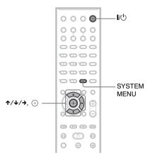
After connecting the AC power cord (mains lead), the demonstration appears in the front panel display. When you press I/U on the remote, the demonstration turns off.
